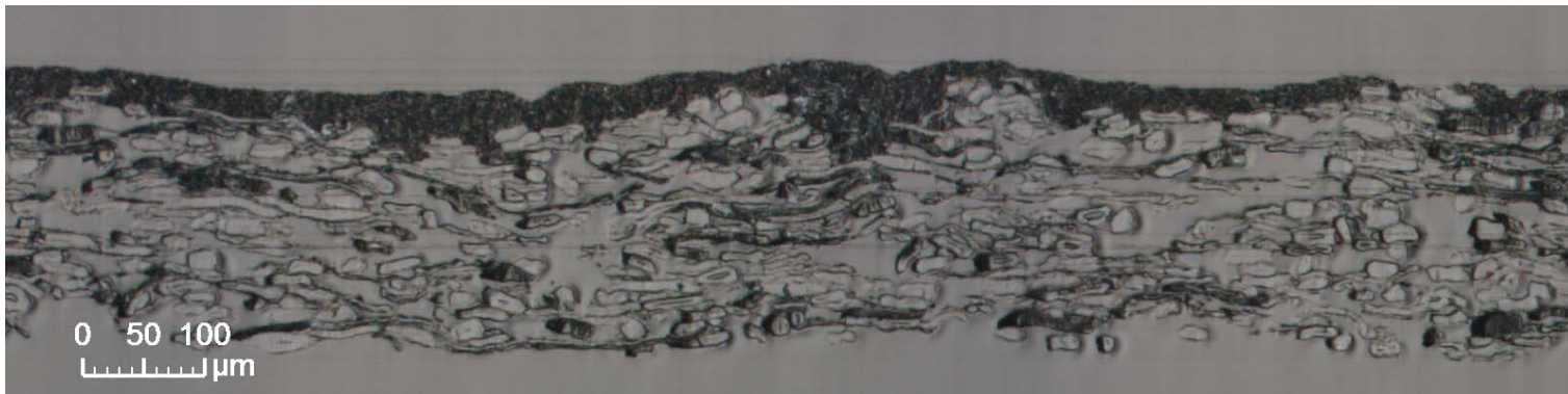
Closed sheet structure (Coating I, carbonate only)
