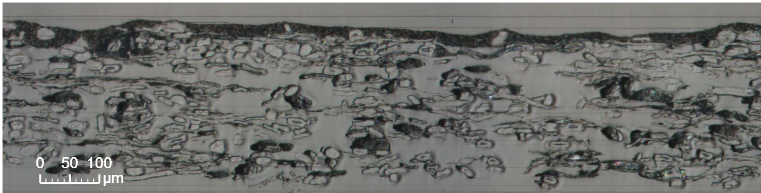
Open sheet structure (Coating II, carbonate and clay)
