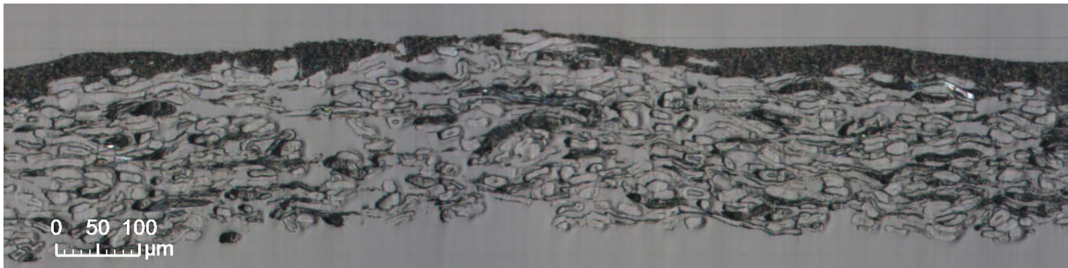
Closed sheet structure (Coating II, carbonate and clay)
